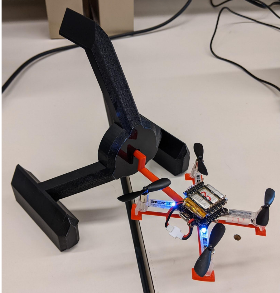
Figure 6. Pitch test stand setup
