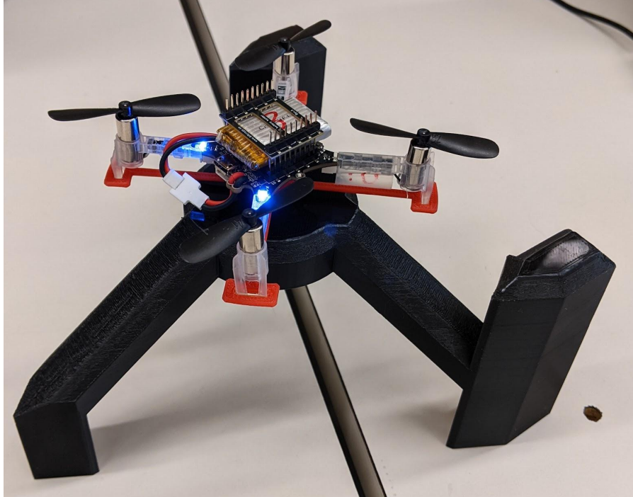
Figure 4. Yaw rate test stand setup
