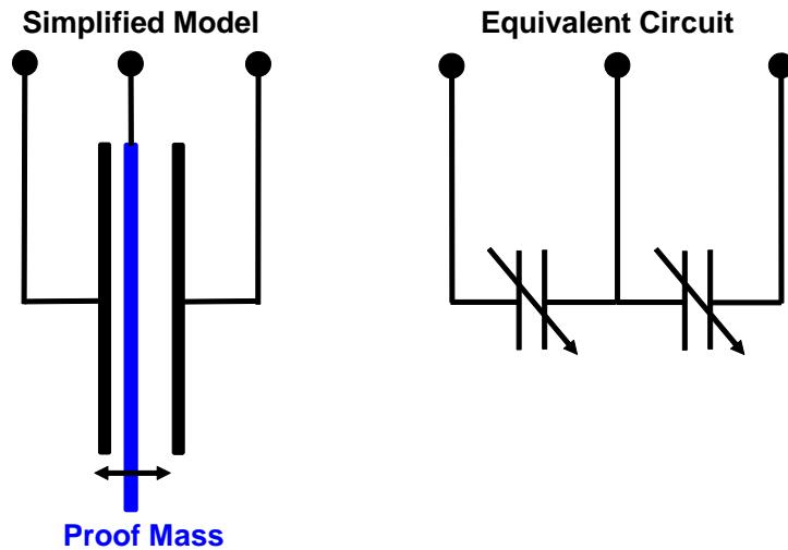
**Figure 2. Simplified Transducer Model and Equivalent Electrical Circuit**
