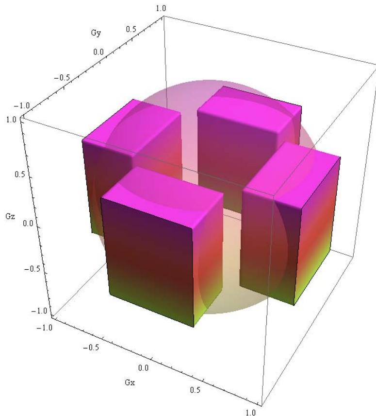
**Figure 9. State Transition Zones for Display Orientation Changes**
