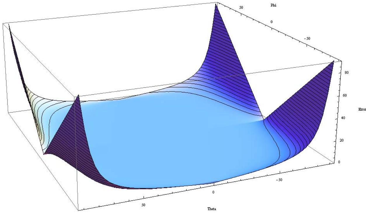
**Figure 4. Roll Angle Error Surface  $|\Delta\phi|$  for  $\mu = 0.01$**
