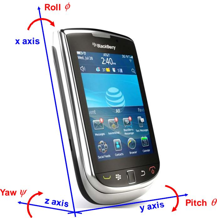
**Figure 3. Definition of Coordinate System and Rotation Axes**
