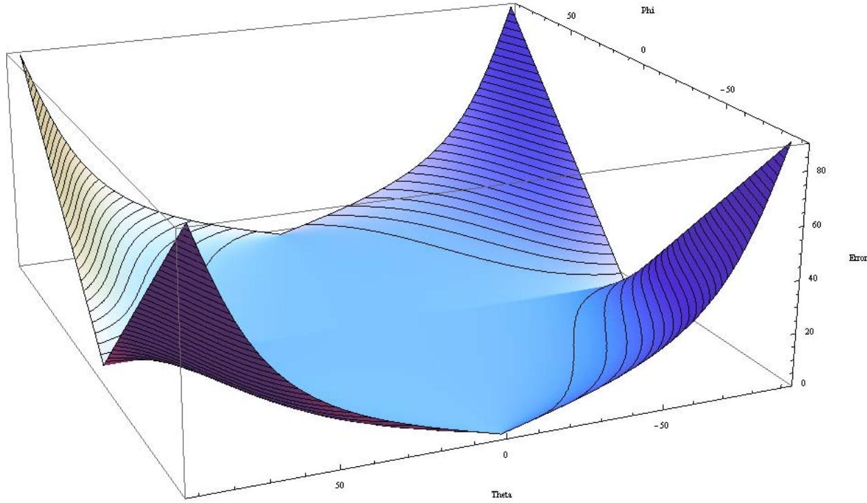
**Figure 5. Roll Angle Error Surface  $|\Delta\phi|$  for  $\mu = 0.1$**
