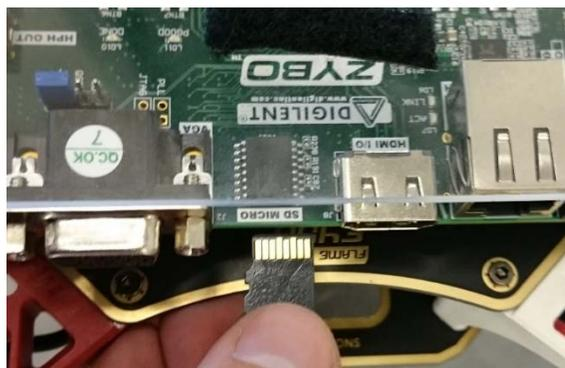
18. Once the card is in, simply turn ON the board and you should see the green Done LED come on (indicating the FPGA was configured successfully) and the program will start executing a few milliseconds after
